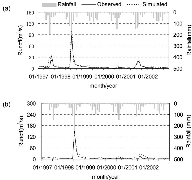
Fig. 3 Monthly hydrological calibration and validation: (a) Xiahui, (b) Zhangjiafeng.
