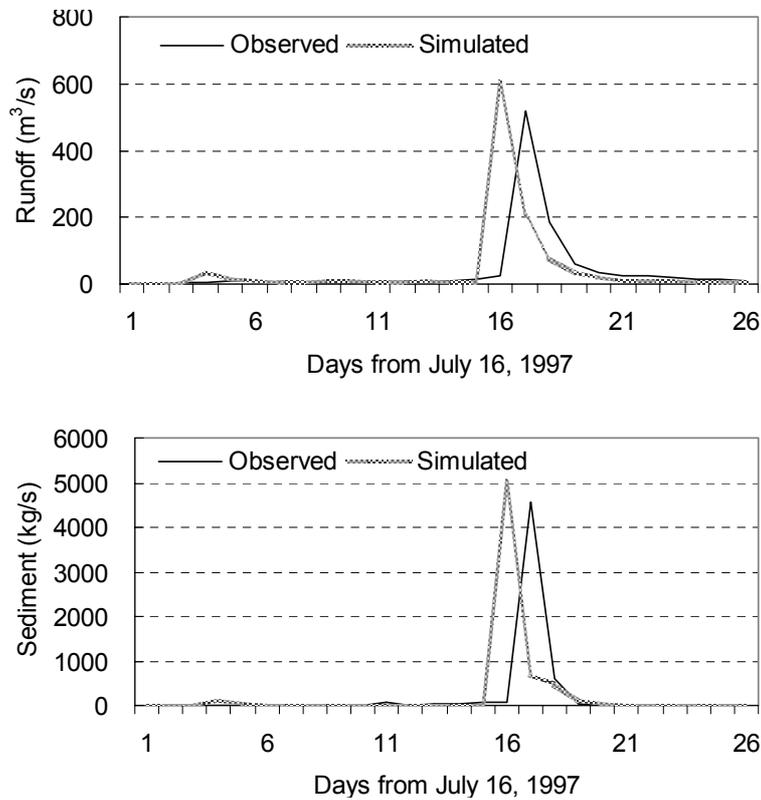
Fig. 6 Daily hydrological and sediment calibrations at the Xiahui station.
